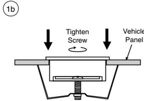
Mounting Hole Diameter: 1.75 in. (45 mm)
