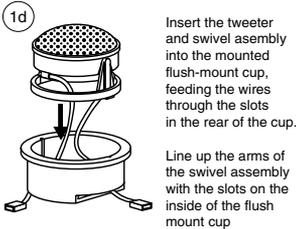
Insert the tweeter and swivel assembly into the mounted flush-mount cup, feeding the wires through the slots in the rear of the cup.
