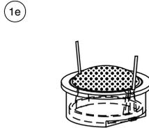
Use two thin metal objects as shown to release the tweeter element from the flush-mount cup.
