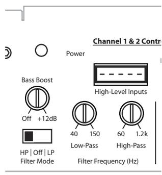
1) **“Filter Mode” Control:** The J2-320.4 employs a 12dB per octave filter for each pair of channels (one filter for channels 1&2 and another filter for channels 3&4). Each of these filters can be configured independently into one of two filter types or defeated completely by way of the three-position **“Filter Mode”** switches:
