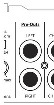
The preamp output signal is not affected by the **“Bass Boost”** processing selected for the amplifier or by any crossover filter selected (if the input signal is full-range, the preamp output will be full-range).
