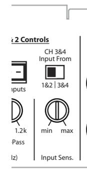
To properly set the amplifier for maximum clean output, please refer to Appendix A (page 12) in this manual. After using this procedure, you can then adjust any or all “Input Sens.” levels downward if this is required to achieve the desired system balance.
