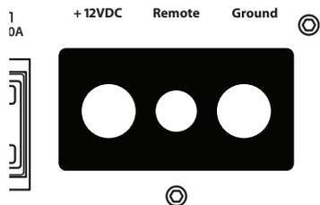
The amplifier will turn on when +12V is present at its “Remote” input and turn off when +12V is switched off. If a source unit does not have a dedicated remote turn-on output, the amplifier's turn-on lead can be connected to +12V via a switch that derives power from an ignition-switched circuit.
