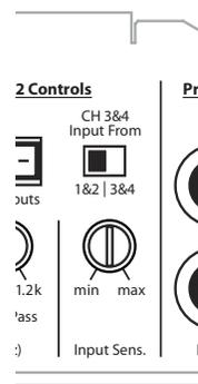
If you wish to feed all four channels by using only two channels of input, set the “CH 3&4 Input From” switch to “1&2” and use only the inputs to channels 1 & 2.
