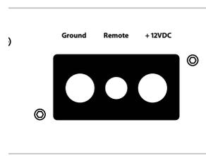
The J2-250.1's “+12 VDC” (positive) and “Ground” (ground) connections are designed to accept up to 4 AWG power wire. 8 AWG is a minimum power wire size for this amplifier.
