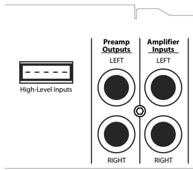
You may run a stereo or a mono signal into the inputs of the amplifier. The amplifier's input section automatically sums stereo signals to mono for the internal amplifier section.
