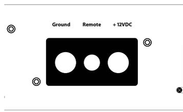
The amplifier will turn on when +12V is present at its “Remote” input and turn off when +12V is switched off. If a source unit does not have a dedicated remote turn-on output, the amplifier's turn-on lead can be connected to +12V via a switch that derives power from an ignition-switched circuit.
