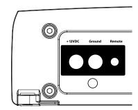
The G2250's "+12VDC" and "Ground" connections are designed to accept 8 AWG - 4 AWG power wire. 8 AWG is a minimum power wire size for this amplifier.
