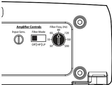
2) **“Filter Mode” Control:** The G1300 employs a 12dB per octave filter. This filter can be configured into one of two filter types or defeated completely by way of the three-position **“Filter Mode”** switch:
