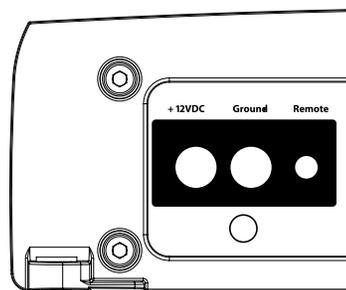
The G1300’s “+12VDC” and “Ground” connections are designed to accept 8 AWG - 4 AWG power wire. **8 AWG is a minimum power wire size for this amplifier.**
