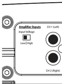
You may run a stereo or a mono signal into the inputs of the amplifier. The amplifier's input section automatically sums stereo signals to mono for the internal amplifier section.
