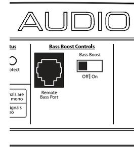
1) **“Bass Boost”:** This switch allows the user to activate a 6 dB boost centered at 48 Hz. The **“Filter Mode”** switch in the **“Amplifier Controls”** section must be in the **“LP”** position for the bass boost to be functional.
