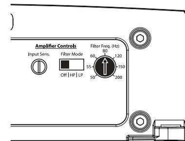
To properly set the amplifier for maximum clean output, please refer to Appendix A (page 12). After using this procedure, you can then adjust the "Input Sens." level downward if this is required to achieve the desired system balance.
