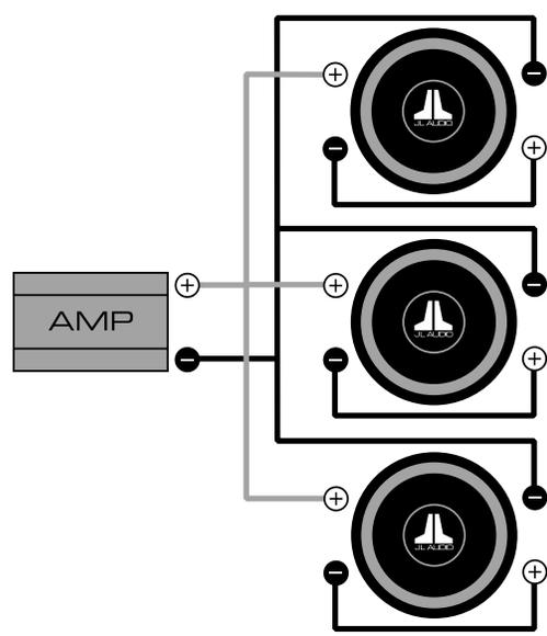
With the coils wired in series and the speakers wired in parallel:
