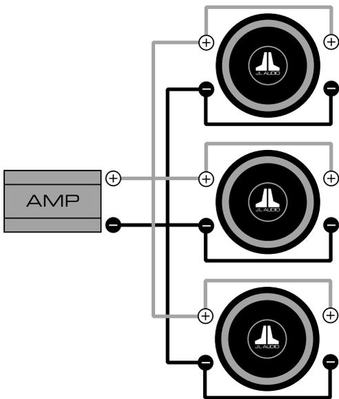
With coils AND speakers wired in parallel:
