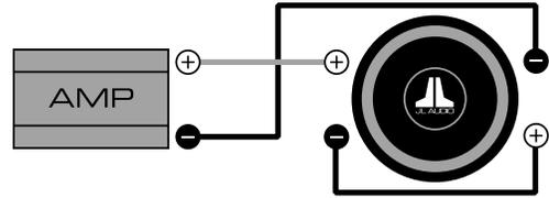
With coils wired in series, a dual 6Ω speaker will present a 12Ω load.
