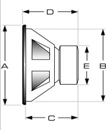
Be sure to allow 0.75 inches (19mm) for pole vent clearance on this driver.
