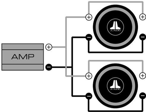
With coils AND speakers wired in parallel:
