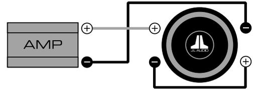
With coils wired in series, a dual 4Ω speaker will present a 8Ω load.
