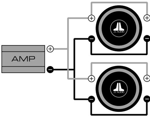
With coils AND speakers wired in parallel:
