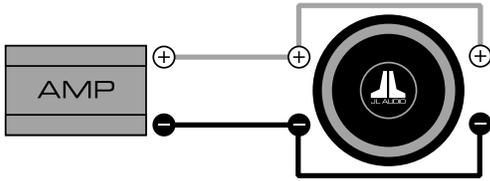
With coils wired in parallel, a dual 4Ω speaker will present a 2Ω load.
