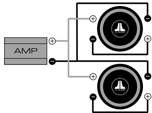
With the coils wired in series and the speakers wired in parallel:
