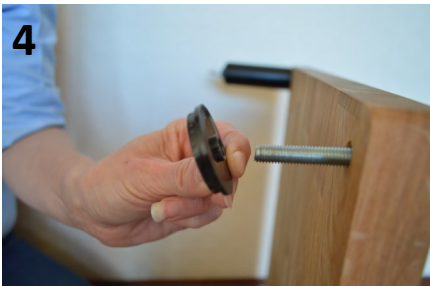
Slide the isolation disc down the stud making sure the protruding lip located on the inner hole is facing the wood
