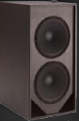
THX-Approved, the KPT-684 is a high-quality subwoofer system that features an advanced low-frequency driver design inside a bass-reflex enclosure for smooth response to the lowest audible frequencies. The system utilizes two 18-inch drivers that gain their amazing 105dB sensitivity through the use of large, geometrically optimized magnet structures and lightweight cones.
