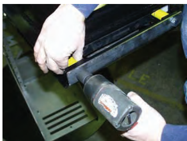
10) Tighten all 4 bolts and torque to 85 ft-lbs.
