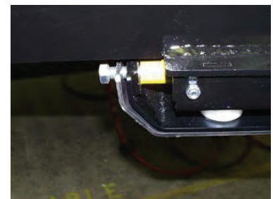
9) Align all 4 bolts before tightening.
