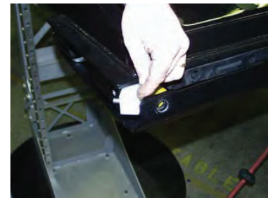
3) Slide spacer blocks into channel.
