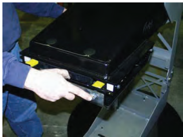
7) Put plate in location using two 9/16-12" bolts opposite corners to hold plate.
