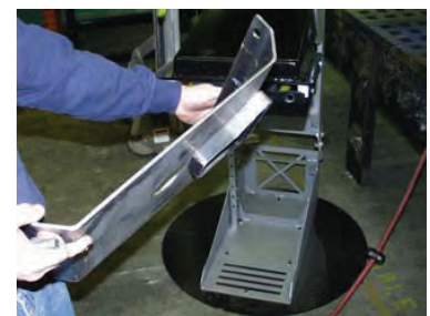
6) Slide Hijacker skid pad (making sure wedge is to rear of box) into place.
