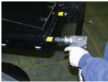
1) Remove four 9/16-12 bolts with 13/16 socket.
