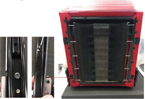
2. Once bottom bolt is hand tightened, then depress track spring to release inner track and slide down to full down position. Apply upward pressure until you hear it click. This will ensure the track is locked. Hand start next two bolts with washers. Torque forward two bolts to 12Nm. Slide inner track up and torque rear bolt to 12Nm.
