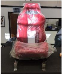
11. Install the seat belt components to the bracket kit, torque to OEM specifications. Install the seat assembly in the vehicle and torque to OEM specifications.
