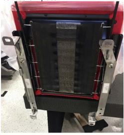
7. Insert 2-M8 bolts through the two rear holes of IB track and hand start nuts.
