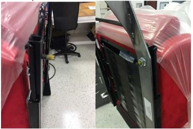
6. Press the towel bar and slide tracks to full rear position. Apply upward pressure until you hear a click to lock tracks in place.
