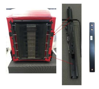
4. Align release lever hole to post on track and press until it is held by clamp. Repeat on opposite side.
