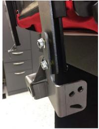
9. Torque all 6 bolts with a 22NM torque wrench.
